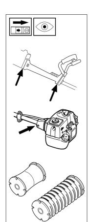
• Check that the vibration damping element is undamaged and securely attached.
